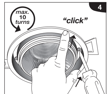
4. Repeat Step 2 by unscrewing second beam direction locking screw.* * Do not use power screwdriver. Do not unscrew locking screw more than necessary (max. 10 turns).
