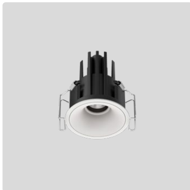
R535 Small Fixed Dimensions D66 x H72mm Cut Out Ø 60mm Watts 11W Lumens <760lm Beam 40°
