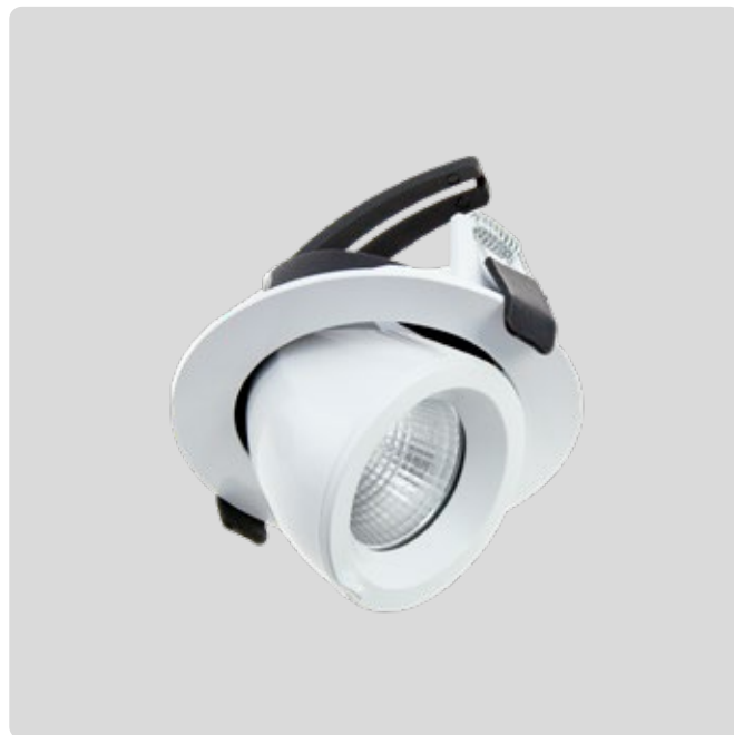
R867 Medium Dimensions D112 x H88mm Cut Out Ø 100mm Watts 9W Lumens <1250lm Beam 50° Tilt -15° to 45° / Rotate 355°
