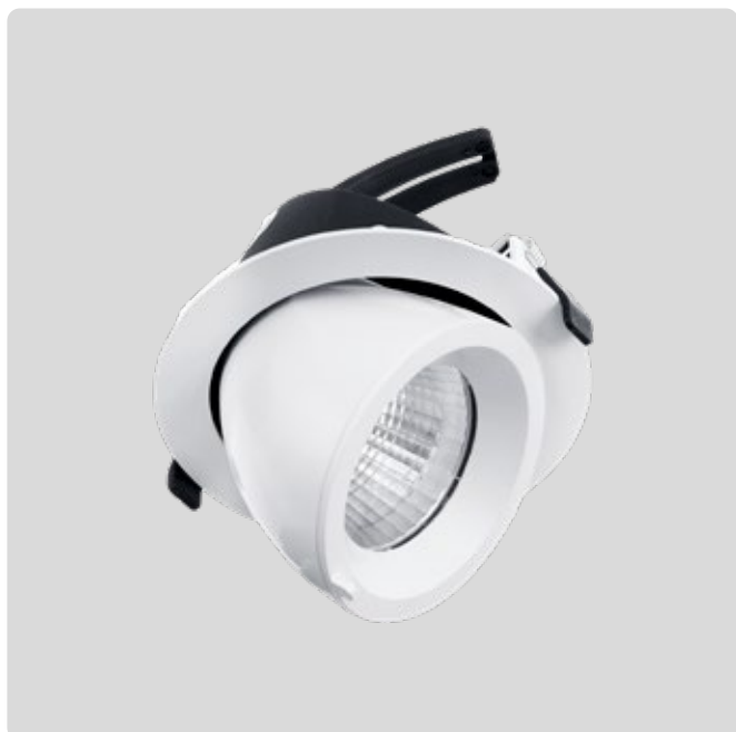
R868 Large Dimensions D162 x H138mm Cut Out Ø 150mm Watts 17W Lumens <2500lm Beam 70° Tilt -15° to 45° / Rotate 355°
