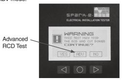
Spark-e-mate briefly displays the ADVANCED RCD TEST mode start up screen.
