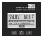
Although the *Spark-e-mate* fascia suggests a test order as per AS/NZS 3000:2007 clause 8.3.4 sequence of tests, the tests can be performed in any order. Apart from overvoltage (>300V AC), there are no wiring transpositions or key presses that can damage *Spark-e-mate*.
