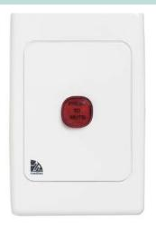
Each RCD shall have an Audible Alarm to highlight that the RCD has tripped. The Audible Alarms shall be the Clipsal ML2000 Series catalogue no. ML2031E08 Series and shall comprise of a mutable two tone audible alarm, flashing red visual alarm, and mute push button labelled "press to mute"
