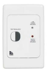
The RCD's shall be the Clipsal ML2000 Series catalogue no. ML2031RC10 Series and shall comprise of 10mA RCD protection, amber load power available indication, red line powder available indication, and an in built test facility.
