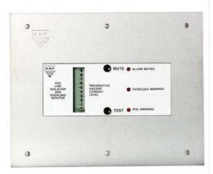
The Line Isolation and Overload Monitors (LIOM's) shall be the Clipsal ESP Series catalogue no. E05 and shall comprise of an 18 segment Prospective Hazard Current (PHC) LCD Bargraph display, mutable two tone audible alarm activated at 5mA PHC and 15A/20A overload current, alarm muted – overload warning – PHC warning amber indicators, and in built test facility.
