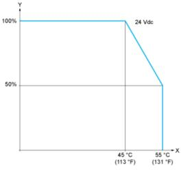
X: Ambient temperatureY: Input simultaneous ON ratio
