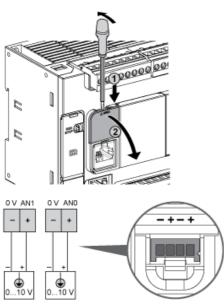
The (-) poles are connected internally.
