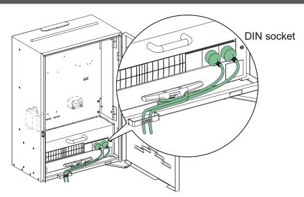
1. Pass the leads through cable protection slide at the bottom opening and tie off before plugging into socket outlet
