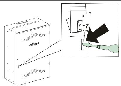
1. Knockout the slot from the inside of door
