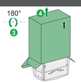
Rotate package by 180° with care and remove carton box
