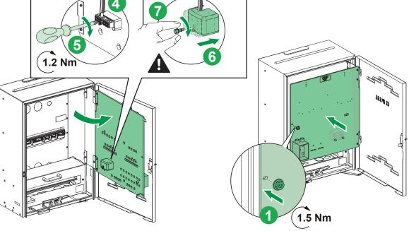
**5.** After wiring, push back the meter panel to its original position and tighten the nut.
