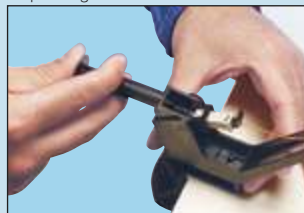
Step 5: Align the fibre
