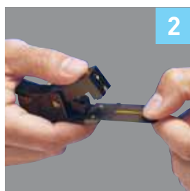
Cleave the fibre
