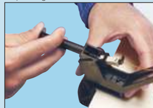
Step 5: Align the fibre
