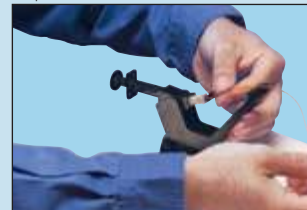
Step 4: Insert the fibre
