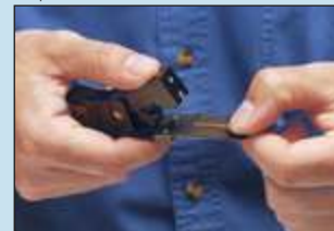
Step 2: Cleave the fibre
