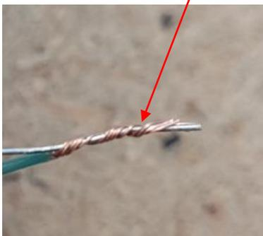
2. Bend one side of the resistor lead over as shown for a clean termination
