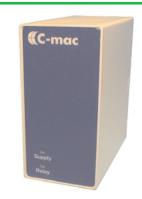
The C-mac<sup>®</sup> module type RP32 meters its own 3-phase supply voltage, and checks that all 3 phases are present and the phase sequence is correct, and in that case the output relay is activated.
